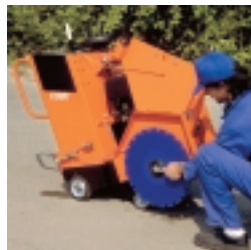
Centrally hinged guard allows quick access for blade changing.
