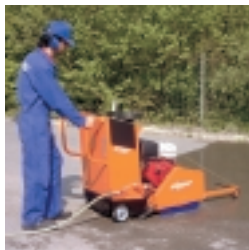
Hydraulic blade raise/lower and self propulsion option.
